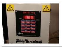
Once dry, place your piece directly onto a shelf in your kiln and fire to Orton Shelf Cone 05 (1020 degrees Celsius). This is the optimum firing temperature for our white earthenware clay.
