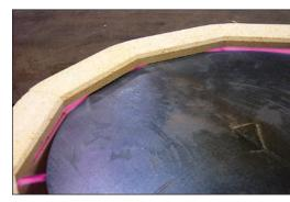
Intentional element contact with the shelf was designed to test the potential for damage from kiln element and controller electrical feedback.
