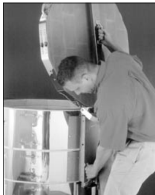
Grasp the two handles shown to lift the lid off the kiln.
