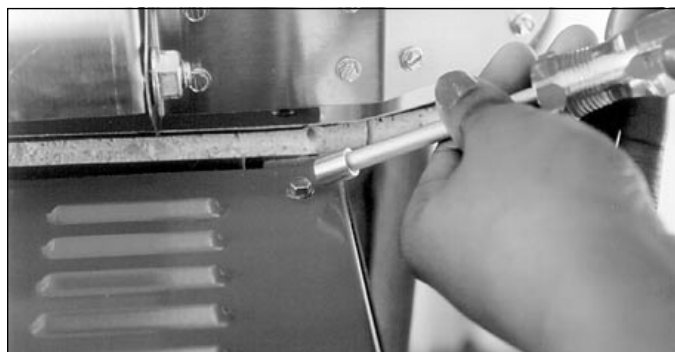
Remove the top two screws from the switch box with a 1/4" nut driver.
