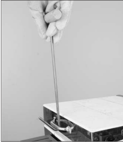
At the end of the venting period, remove the post with a Lid Lifter and hot glove (available from Paragon).
