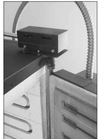
The door safety switch turns off the elements when the door is opened.
