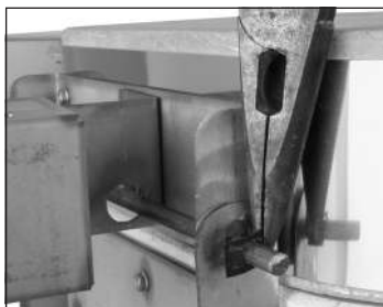
Grab a spring clip with needle nose pliers. Then slide the clip off the shaft.
