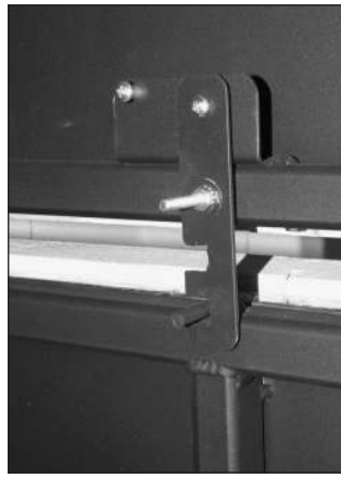
The swing-away vent latch in the vented position
