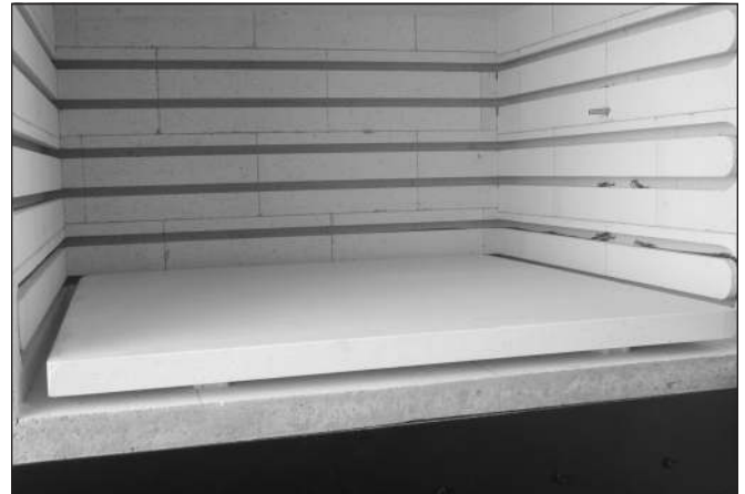
A shelf on ½" (12.5 mm) posts. The space between the kiln bottom and the shelf improve the heat distribution through the glass.
