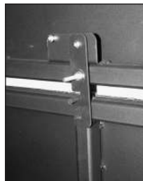
Keep the swing-away vent latch in the closed position when the kiln is not in use.
