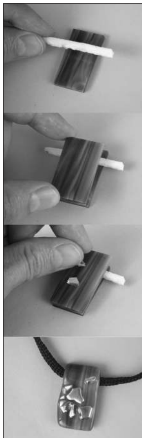
You can use a strip of \frac{1}{8} " thick fiber paper to make a channel for a cord in a glass pendant.
