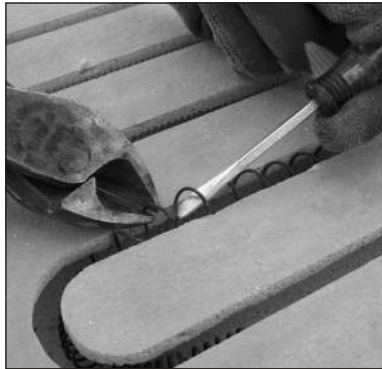
Shown outside the groove: Cut the element after stretching it.
