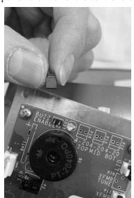
Remove the 2-pin jumper plug from the connectors labeled BUZZ ENABLE to silence the beeping alarm. You will find the connectors on the back of the controller.
