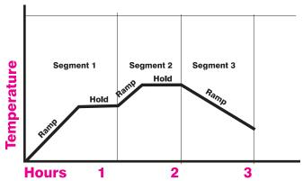
Here is a simple 3-segment program. Segments 1 and 2 each have a hold. Segment 3 is a controlled cooling segment.
