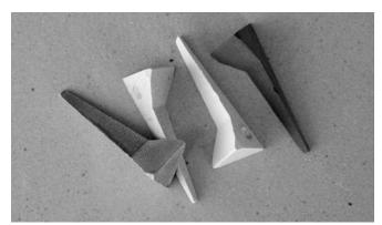
Orton self-supporting pyrometric cones.
