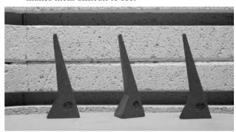
The heating element in the background should be lined up with the lower part of the witness cones. If the element is too high, the tips of the cones will disappear from view when they bend.
