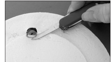
Use a pocket knife to remove embedded glass from the base.
