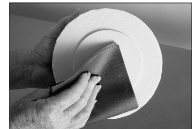
Sand off a damaged coat of glass separator before applying a new coat.
