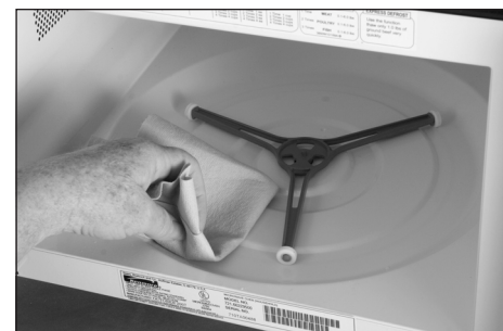
Clean the rollers and track for the smoothest rotation of the tray.
