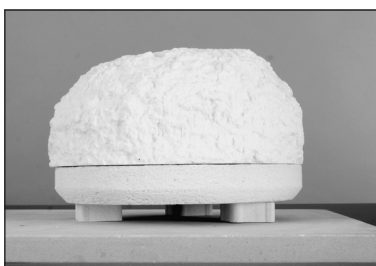
Place 3 ceramic posts between the kiln and a heat-proof surface.
