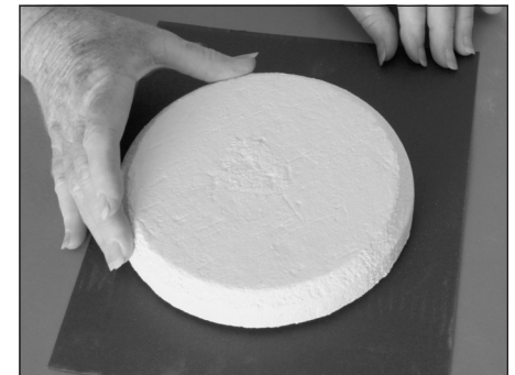
Sanding the base to remove minor gouges.
