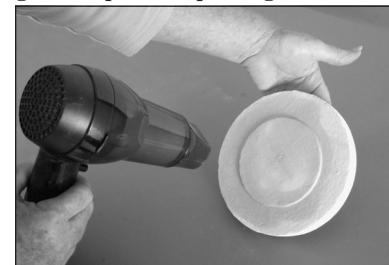
Drying the glass separator with a hair dryer.
