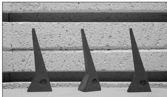
Line up the heating element with the lower part of the cones.
