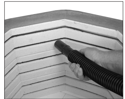
If you vacuum with a plastic nozzle, do not let the nozzle touch the fragile firebricks.
