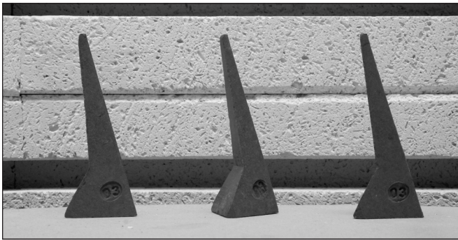
Self-supporting cones on the kiln shelf verify that the clay and glazes receive the correct amount of heat work.
