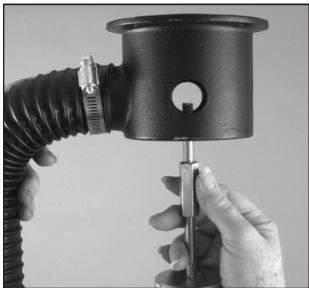
Adjusting the Orton Master Vent for installation under the kiln.
