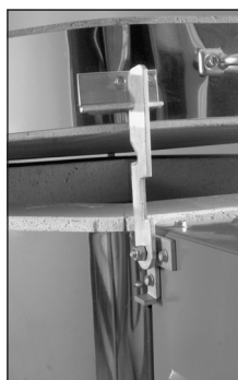
Prop the lid in the extended position when firing ware draped with lace. Lower the lid when all smoke disappears.
