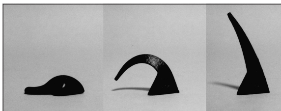
Self-supporting cones: Left, over-fired or "puddled"; Center, fired to maturity; Right, under-fired.
