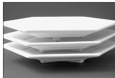
You can use stilts to separate a stack of horizontal plates. But do not stilt soft glazed pieces. Test if you are not sure.
