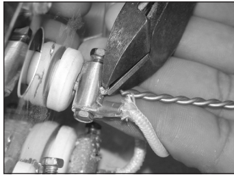
Install the element connector flush against the porcelain insulator. After tightening, cut off excess length.
