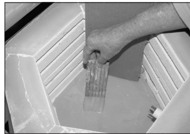
Protect the elements when you apply kiln wash to the brick bottom.
