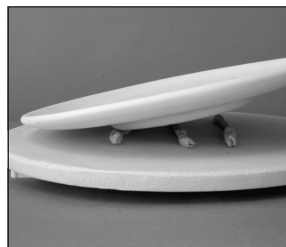
Separating the plate from the shelf helps to prevent cracking of the ware.
