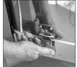
Remove the screws that hold the twist latches to the kiln bottom.
