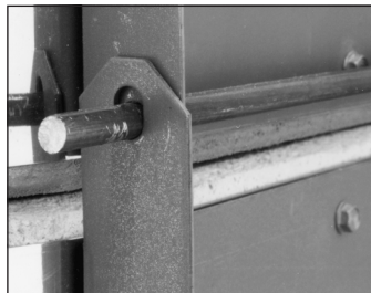
Install the hinge so that with the lid closed, the rod rests in the bottom of the slotted hole as shown here.
