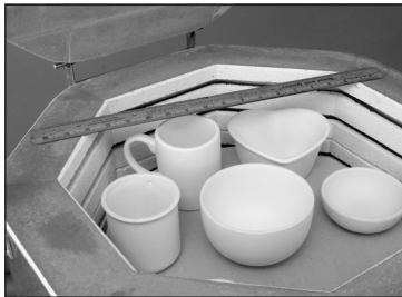
Lay a ruler across the top of the kiln to make sure the ware is not too high.
