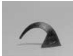
**The cone did not bend far enough:** Use a 00\_\_ Cone Offset number for a hotter firing. (About 0025 for the cone at right.)
