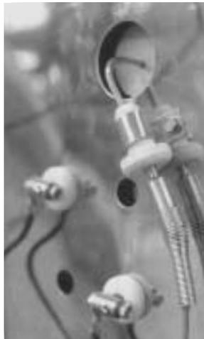
low the thermocouple, including its spring, to touch anything metallic, such as a heat shield.
