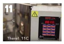
Your new thermocouple should now read room temperature. Begin a test firing and check the temperature increases. If you install the thermocouple the wrong way round, it will read incorrect temperatures and you will see the temperature on the display decrease as the kiln heats up
